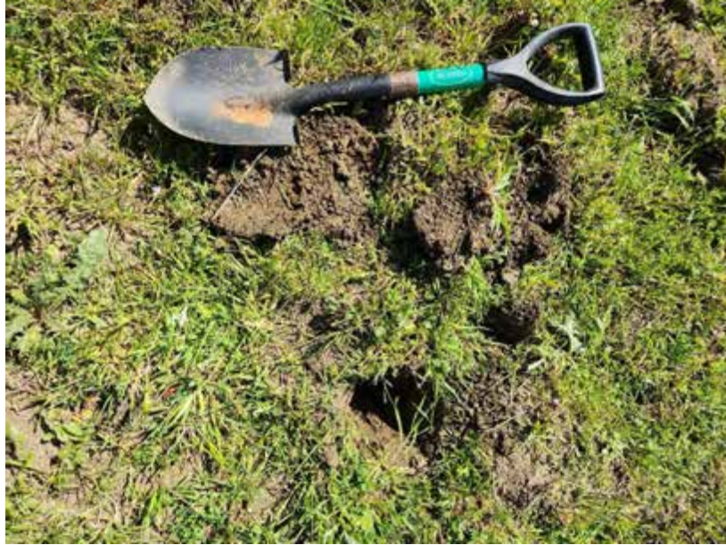
Photo of test pit showing upland soils (sandy loam, oxidized, not saturated)
