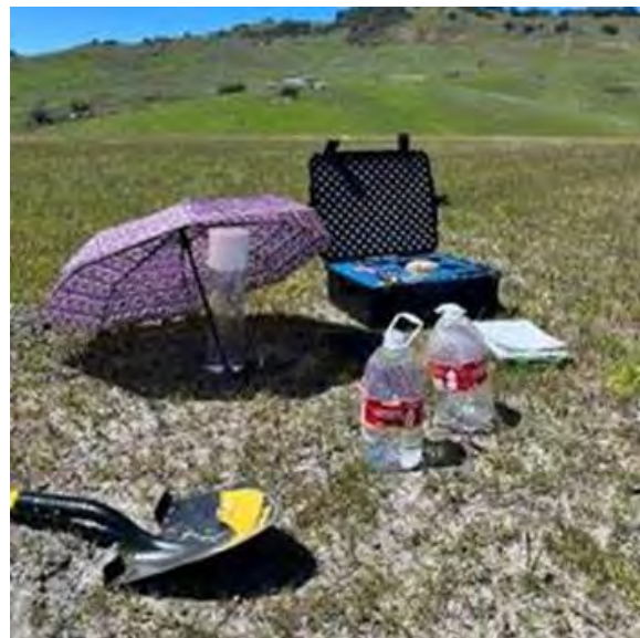
Photo 2.6.3-1: Infiltration Field Set-Up
